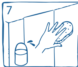
Remove the overflow glue with damp sponge.
